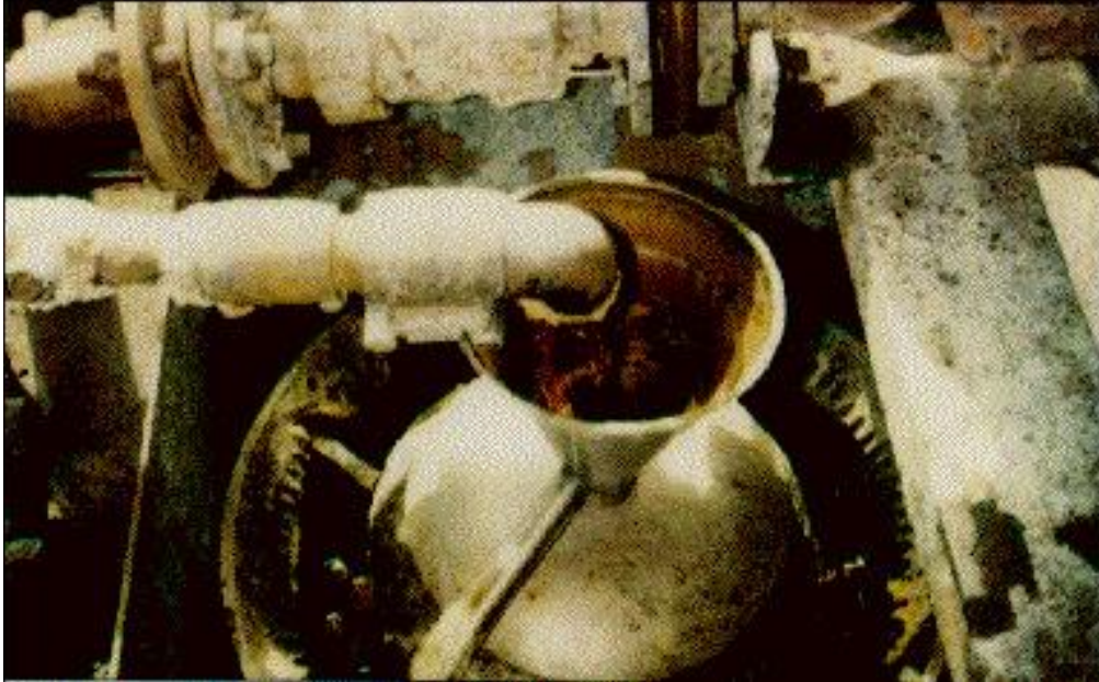
Distribution cup used to distribute sodium ethyl xanthate evenly through flotation tanks.
