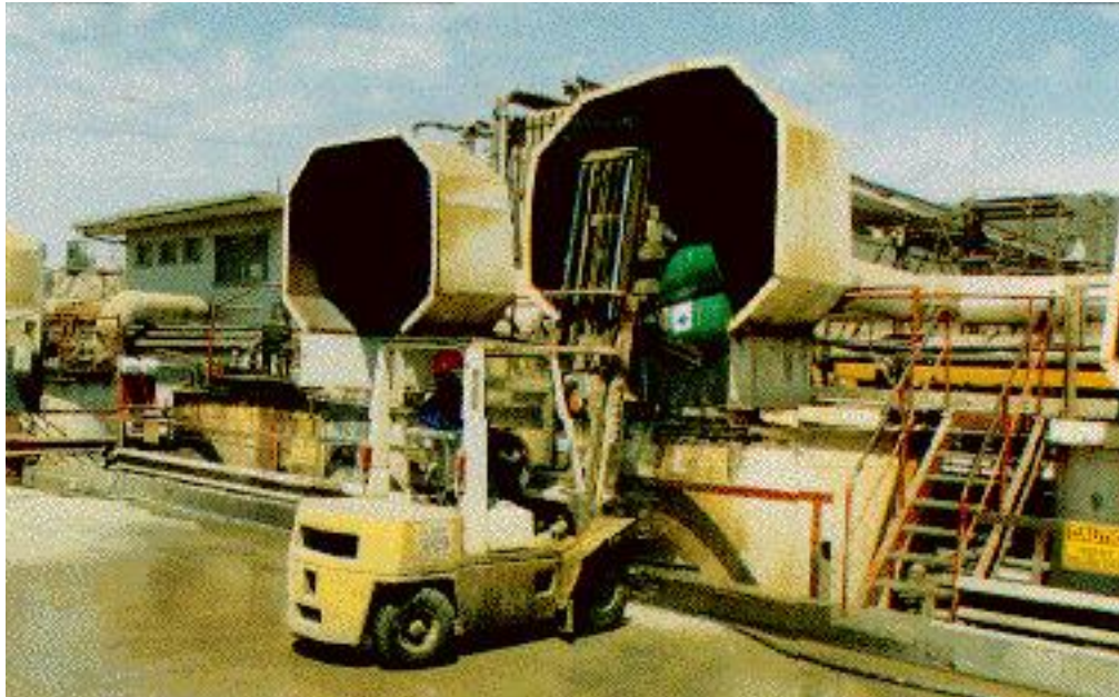
Mixing area showing the emptying of drums containing sodium ethyl xanthate.
